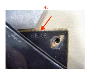
Reposition the assembled base to the bottom of the chair seat. Note that the stamped "REAR" in the swivel must face to the rear of the chair seat. Reinstall the (4) 7/16" hex head bolts and tighten securely.
