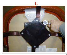
Lay chair upside down on a clean, smooth surface. Rotate chair base to expose the (4) hex head 7/16" bolts that secure the swivel to the chair seat. Remove these (4) bolts.
