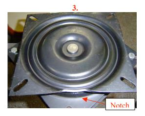
Reinstall swivel to base plates and square tubular leg frame. Note that the side of the swivel with the notch must face opposite from the legs.
